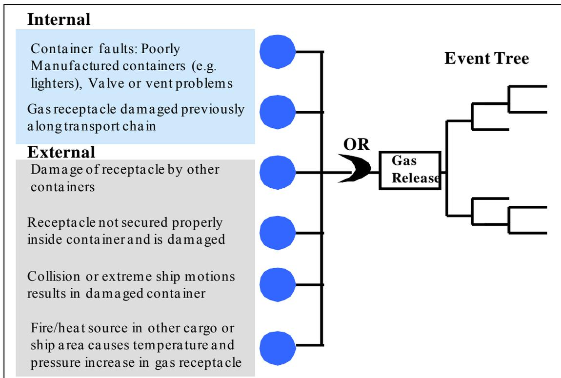
**Figure 14: High level causes for release of gas.**
