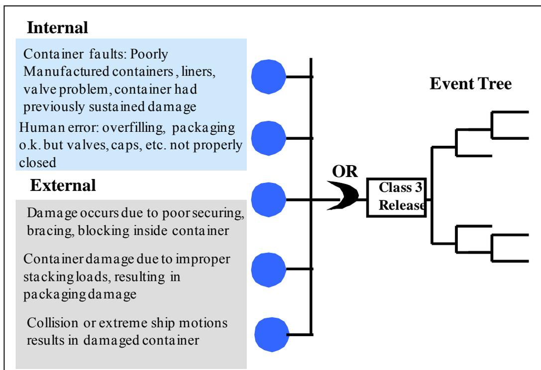
Figure 15: High level causes for release of Class 3 Flammable Liquids.
